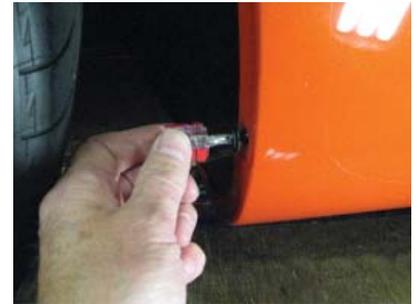
2. Using your flathead screwdriver or trim tool, remove the plastic push-pin fastener from the wheel-well liner. Remove center pin first and then the housing can be removed.
