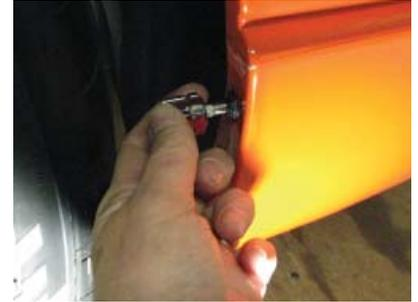
2. Install the phillips fastener through the stone chip guard hole and into the wheel well lip hole. The cage-nut in the wheel well housing will allow minor adjustment and alignment as needed.
