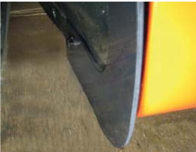
4. Install the stone chip guard by inserting the push-pin housing back into the wheel well liner hole. Push the pin into the fastener to lock.
