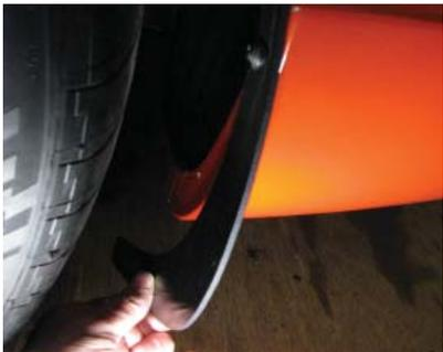
4. Rotate the stone chip guard away from the wheel well lip so that the self-adhesive discs can be seen on the reverse side of the guard. Clean the exposed wheel well lip with alcohol and cotton cloth.
