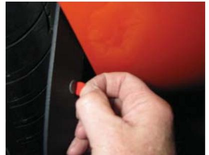
6. Carefully rotate the stone chip guard to the wheel well lip, aligning to your masking tape guide. Once in position, apply pressure to the stone chip guard to adhere the surfaces. Phillips fastener can now be tightened.
