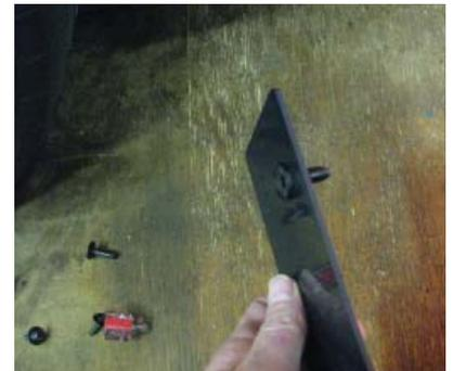
3. Install the push-pin housing (without the pin inserted) in the large hole of the stone chip guard.
