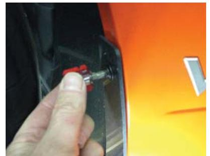
5. Reinstall the two phillips fasteners through the stone chip guard and into the wheel well lip. The cage-nuts will allow minor adjustment and alignment as needed.
