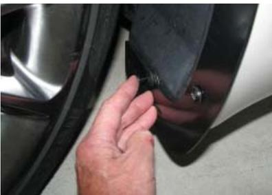
6. Once seated, push the pin into the fastener to lock. Note; The five oval shaped holes at the bottom of the stone chip guard allow air-flow into the sill of the Viper.
