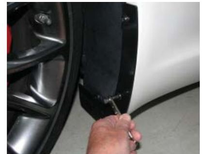
3. Fasteners may be tightened, but be careful not to over-tighten or strip.
