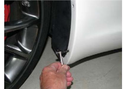
2. Align the upper two ¼" round holes of the guard with the two open holes of the wheel well lip. Install by re-using the torx fasteners. The cage nuts will move as necessary to line-up with the holes in the stone chip guard and wheel well lip.
